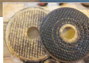
A split-up CJC™ Vri Filter Insert disk, revealing how the contamination is absorbed into the cellulose
