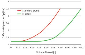
*Chart: Comparison of filtration capacity between a standard filter media grade and the high-capacity H grade.*
