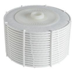
Depth filter modules make it possible to handle large filter areas in a simple manner and have been used in various food & beverage applications for many years. Filtration with such modules is carried out in an enclosed system (DISCSTAR<sup>™</sup>). The filter medium used in lenticular modules is a depth filter sheet. A combination of surface, depth and adsorptive filtration mechanisms lead to a high filtration performance. Depth filter products represent a cost-effective filtration solution.
