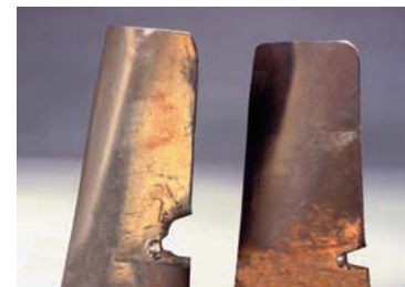
Severely damaged turbine blades seriously affect power output.
